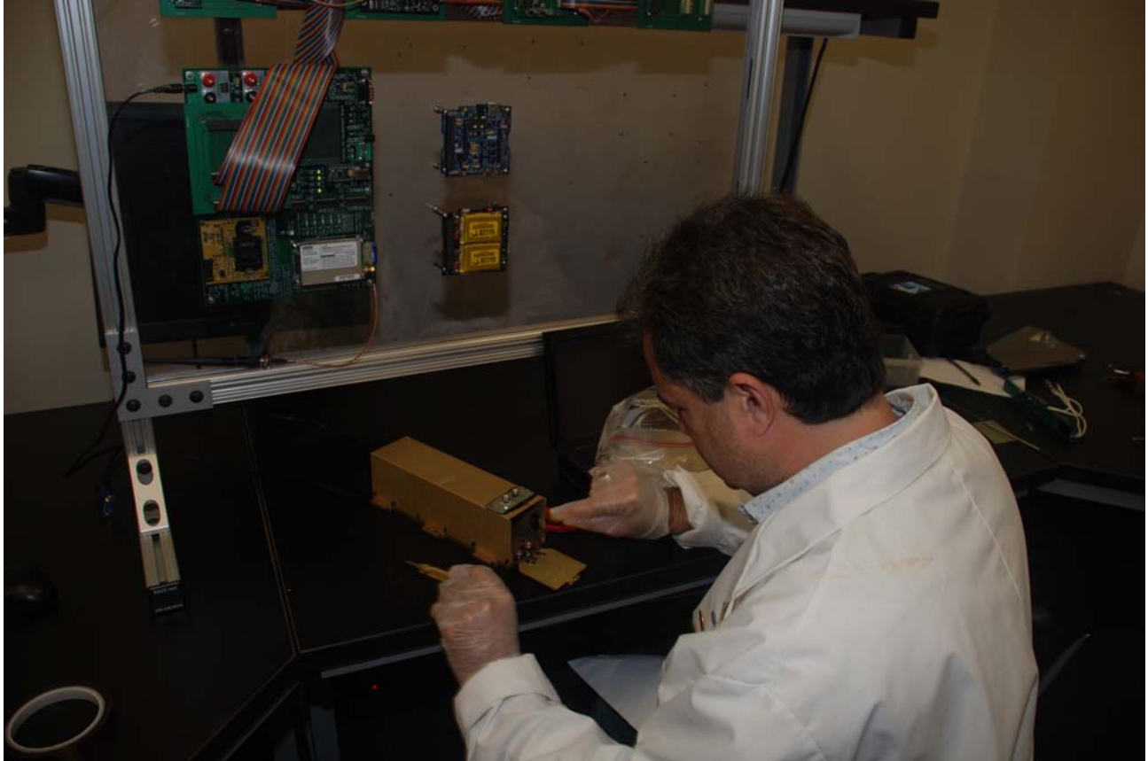
Dr. Malphrus examining one of the Morehead-Rome Femtosat Orbital Deployers (MRFODs) that are installed in the EduSat microsatellite and will ultimately eject femtosatellites developed by students at Morehead State University and the University of Rome
