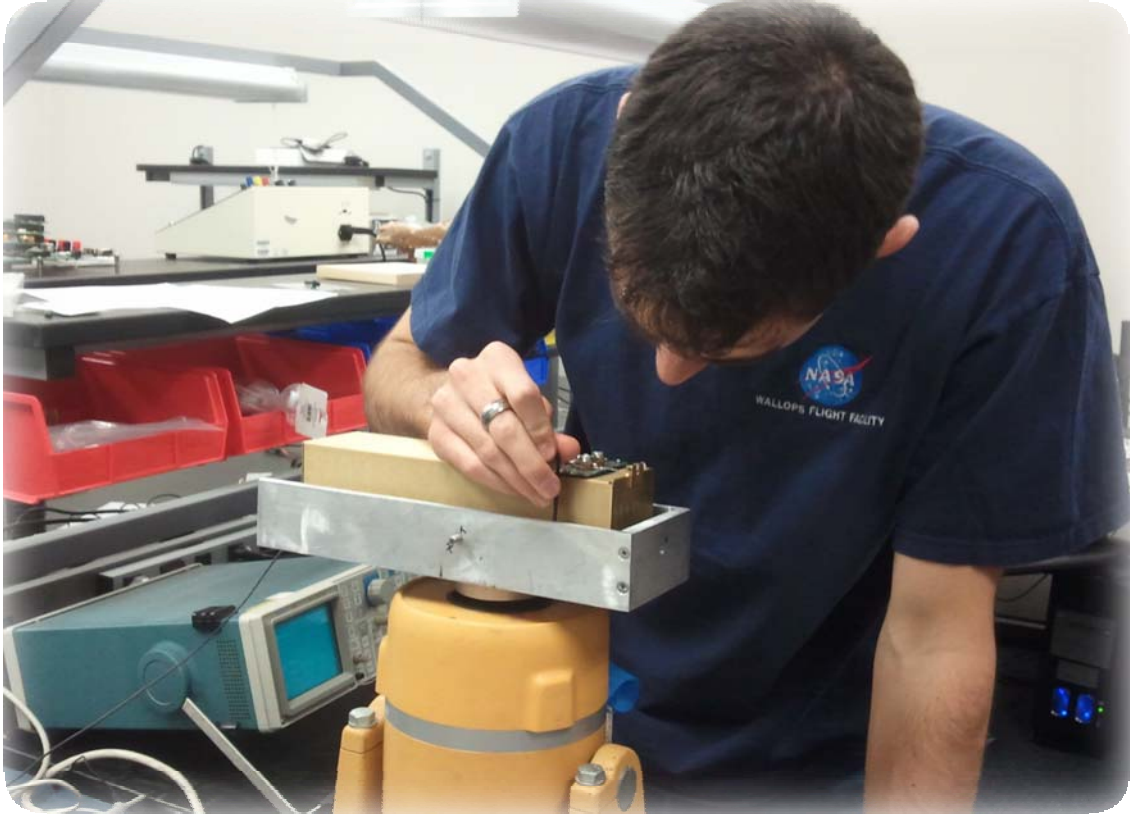
Tyler Rose, a Space Science Student, Prepares One FOD Unit for Vibration Testing
