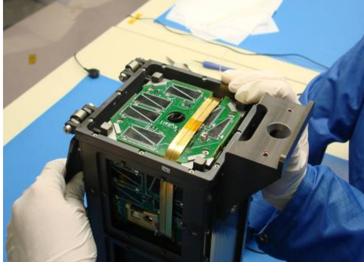
Figure 4: KySat-1 CubeSat in a P-POD
